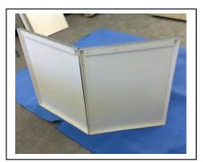
Next, start to assemble the side panels (the end with the holes to top, flat side inwards), join panel together with nuts, bolts and washers provided. It is best at first to leave the screws loose for each section until all the sides are together and then go round and tighten them. This is the last opportunity to check you are happy with the position of the pool, before you put the liner and water in.
