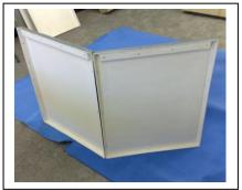
Next, start to assemble the side panels (the end with the holes to top, flat side inwards), join panel together with nuts, bolts and washers provided. Use 2 washers per bolt: ensure the fibreglass is sandwiched between two washers. It is best at first to leave the screws loose for each section until all nine sides are together and then go round and tighten them. This is the last opportunity to check you are happy with the position of the pool, before you put the liner and the water in.
